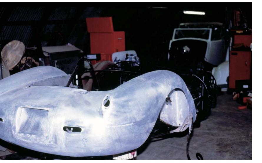
the aluminum body was riveted to that *little strip, to the chassis.*
